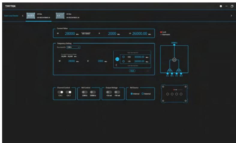
\*If the device cannot be recognized normally, please confirm the network environment settings. domain must be set to 192.168.100.xxx. (If the IP address of the device and PC is assigned by DHCP, this step can be skipped.)
