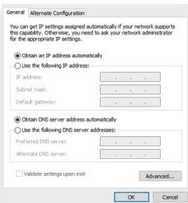
If no DHCP function supported, the static IP needs to be configured manually. Please set the control terminal IP to 192.168.100.xxx.
